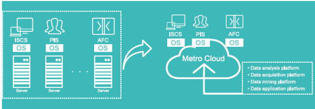
MACS-SCADA Integrated Supervisory Control System (ISCS) Based on Cloud Platform
