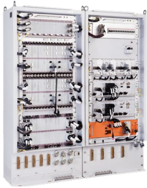
Train Control Vehicle System (ATP)
