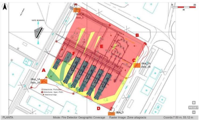
Figure 6. Initial fire detectors coverage
